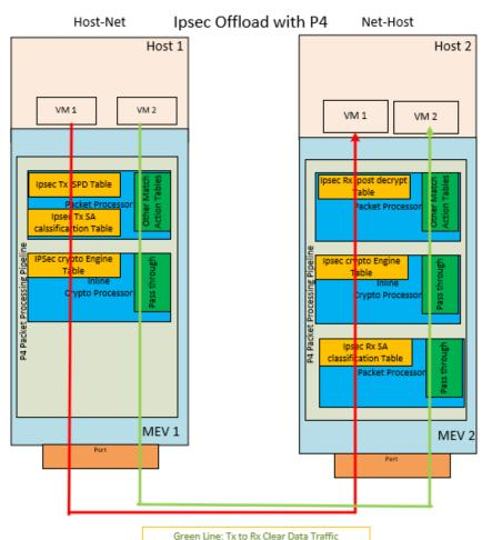
Green Line: Tx to Rx Clear Data Traffic Red Line: Tx to Rx IPSec offloaded Data Traffic
