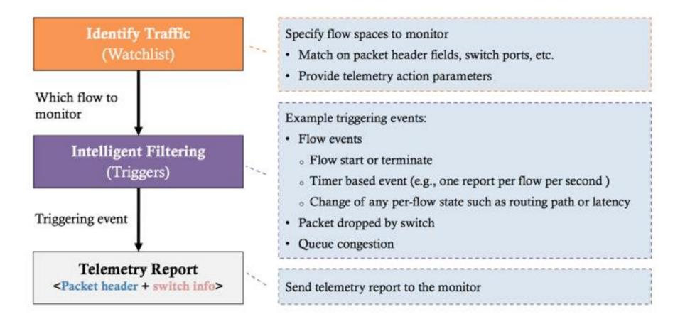
Three logical functions (above) can be placed at different network locations (**different INT modes in next slides**) to best meet the requirement and deployment constraints, such as live data packet modification.
