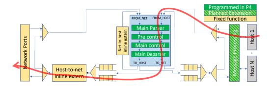
Figure 6. Host to network packet path
