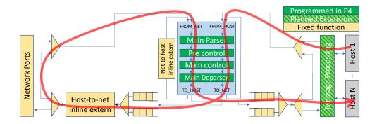
Figure 8. Host to host packet path
