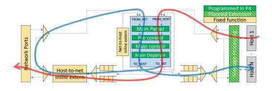
Figure 7. Host to network packet path, with mirror copy to a different host
