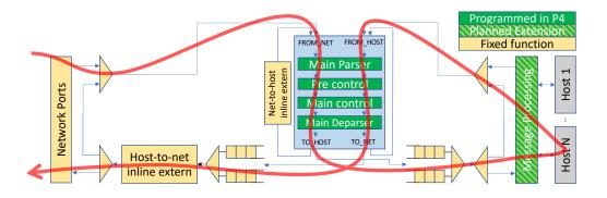
Figure 9. Port to port packet path
