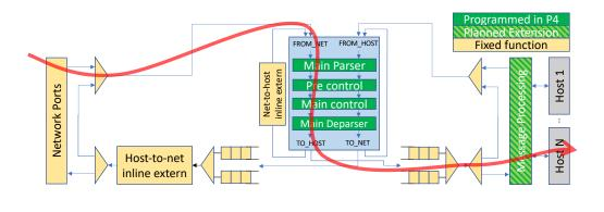
Figure 4. Network to host packet path
