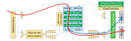
Figure 5. Network to host packet path, with mirror copy to second host
