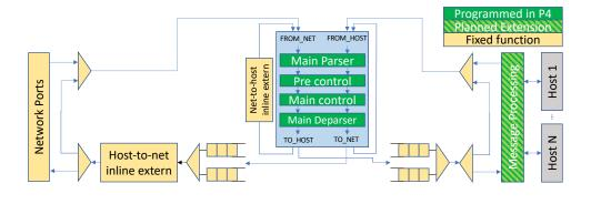
Figure 1. Programmable NIC Architecture Block Diagram
